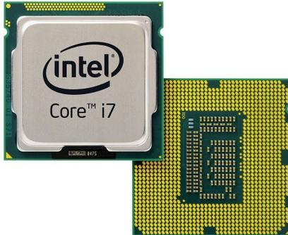
A processor or microprocessor is built into a microchip that has memory and other components built into it. The microchip itself is often referred to as the 'processor'. If there is more than one processor built into the microchip, then the microchip is referred to as the 'processor' and processors built into it are referred to as cores.
