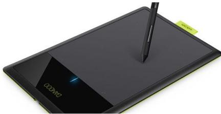
Graphics tablet or a graphics pad is a flat rectangular pad between 6 and 20 inches wide. It works with a stylus which you move along the surface of the pad to produce drawings in the computer. There are several types of stylus. One, the puck, is small rounded device with cross-hairs for tracing lines accurately and with a number of buttons. The stylus can also be pen-shaped. A graphics tablet is used mainly for computer-aided design and drawing.
