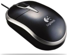
The mouse is the most widely used pointing device. Some have the ball underneath that moves when you move the mouse, resulting in a similar movement of the pointer on the screen. A optical mouse detects movement using light instead of a ball.
