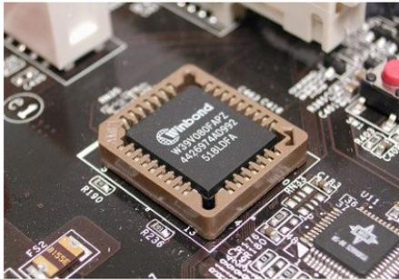
Read only memory can also be accessed in random order, but the data in it cannot be changed. ROM is intended for permanent data, necessary for the operation of the computer system. ROM is non-volatile, which means that it retains what is stored in it when the computer is turned off.
