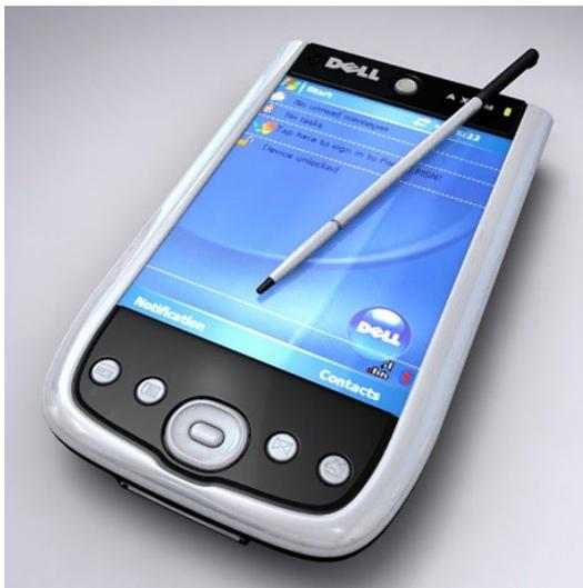
A handheld computer or Personal Digital Assistant (PDA) or palmtop can fit in one hand or in your pocket, but it is too small for general work. A PDA usually has a touch sensitive screen. Although PDAs can be temporarily attached to a Keyboard, you cannot comfortably type a long document into a PDA.
