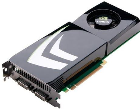
The graphics card which is also known as video card or display card is housed within the system unit, and controls the signals going to the monitor screen. Higher quality cards can produce very clear graphics very quickly. Some computer games demand advanced display cards and high-quality monitor screens.
