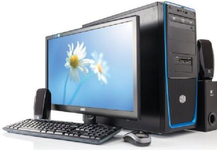
A desktop PC usually has these basic components: a monitor, a keyboard, a system unit and a mouse.
